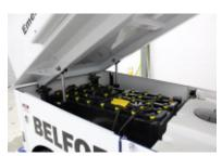
Studies have shown that the largest contributor to poor indoor air quality in enclosed ice arenas are the ice resurfacer and the edger. Typically fuel-fired, these two pieces of equipment emit carbon monoxide (CO), nitrogen dioxide (NO<sub>2</sub>), and particulate matter (PM), which can negatively contribute to health issues. At the Double Ice Complex, all ice maintenance equipment is electric, helping to ensure a high quality indoor environment for the community.
